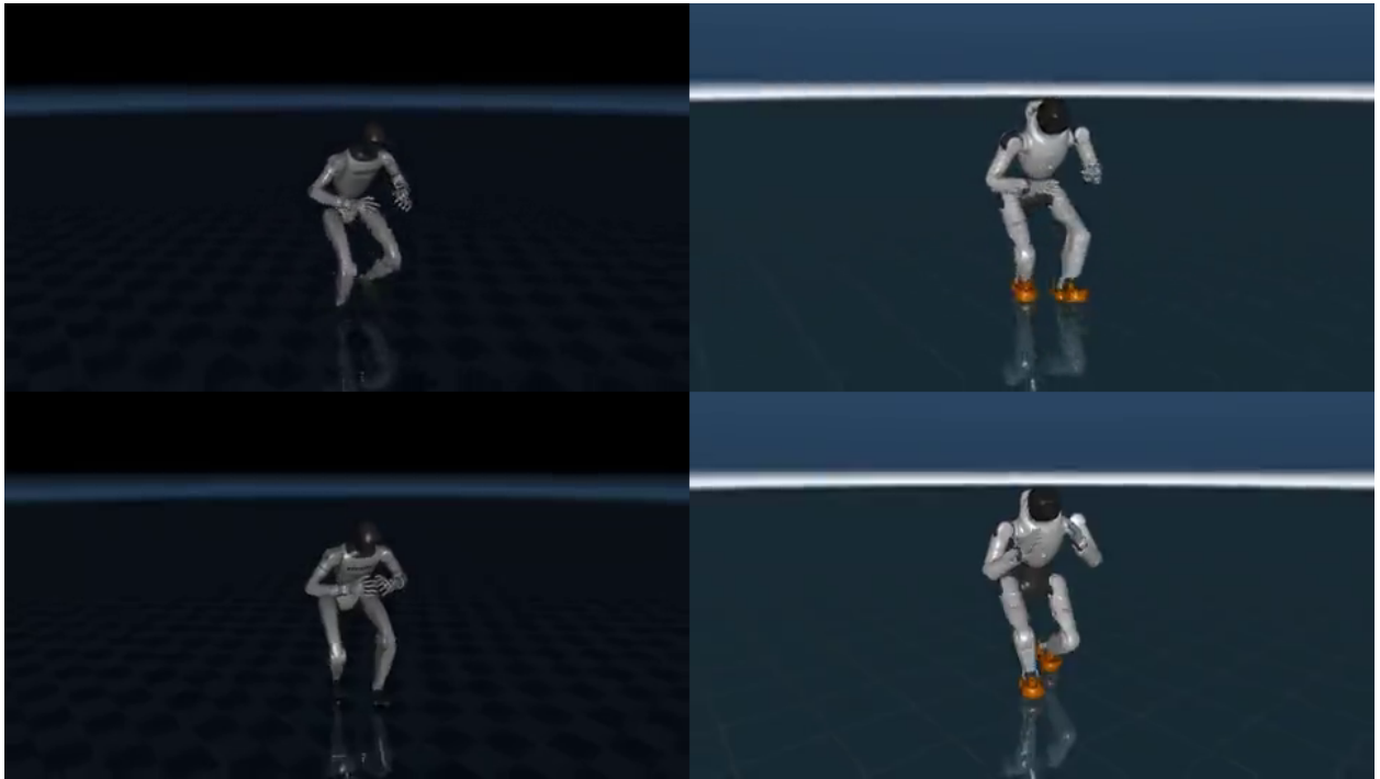
Figure 9: F9c — Crouch walk (hip 0.55 m). A capability neither native X2 planner had; inherited from the source core’s crouch template for free. Depth saturates at the source corpus’s floor (§9).
